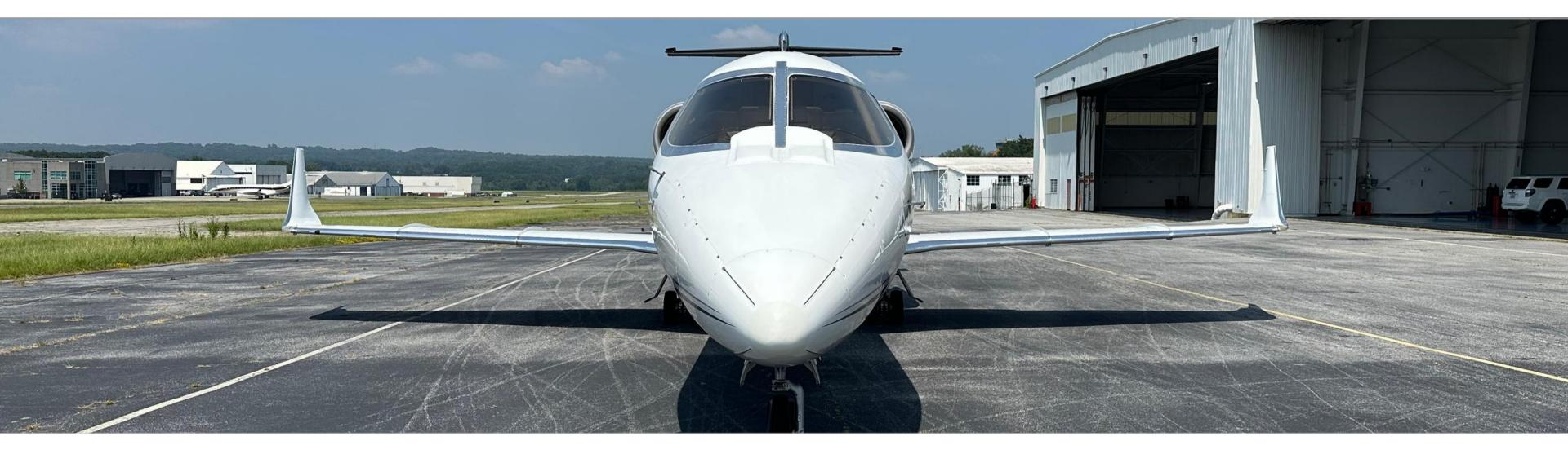
THE 1994 LEARJET 60 IS A MID-SIZED BUSINESS JET REPRESENTING A SIGNIFICANT ADVANCEMENT IN THE LEARJET SERIES. BOMBARDIER AEROSPACE PRODUCED THIS AIRCRAFT WITH A SLEEK DESIGN AND IMPRESSIVE ENGINEERING. RENOWNED FOR ITS SPEED AND EFFICIENCY, THE LEARJET 60 BOASTS TWIN PRATT & WHITNEY PW305A ENGINES THAT PROVIDE EXCEPTIONAL PERFORMANCE. THIS AIRCRAFT HAS A RANGE THAT EASILY EXCEEDS 2,000 MILES AND CAN CLIMB AS HIGH AS 51,000FT.
